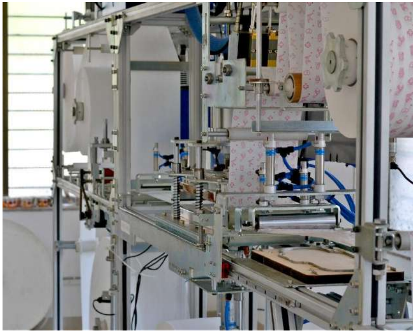
Swacch automatic sanitary napkin-making machine at Saral Design's factory. Photo credit: Sharanya Hariharan.
